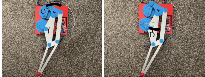
Fig. 6. Trajectories of Points C (left) and D (right) with a 270 degree offset. It can be noted that regardless of the offset, the trajectories geometry remains the same.
